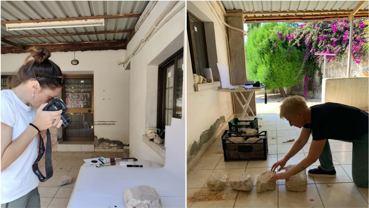
Figure 3. Macroscopic analysis and documentation of mudbrick samples during fieldwork activities (EARTHERITAGE Project Archive).
