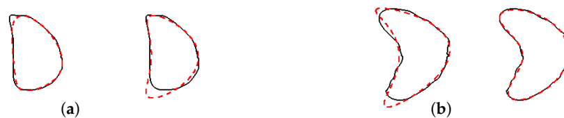
Figure 13. The solid black curves are ground truths and the dashed red curves are the model curves found by the method (in each figure from the left to the right: CS and CC model). The two comparisons show some cases in which a different model gives a result better than the other one. (a) CS model ( d_m = 0.39 mm, d_H = 2.45 mm, DSC = 97.2\% ) and CC model ( d_m = 0.66 mm, d_H = 4.06 mm, DSC = 93.3\% ). (b) CS model ( d_m = 0.68 mm, d_H = 2.92 mm, DSC = 93.8\% ) and CC model ( d_m = 0.26 mm, d_H = 1.45 mm, DSC = 98.0\% ).
