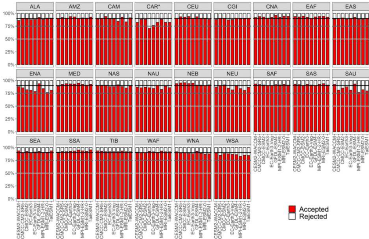
Figure 3.13: Results of the AIC bootstrap approach for the validation of the GCMs. The panels indicate the IPCC zones, while the bars refer to the nine GCMs analyzed. The red color indicates the percentage of pixels where there is not enough evidence to reject the null hypothesis that the GCM outputs can be extracted from the same copula as the reference data
