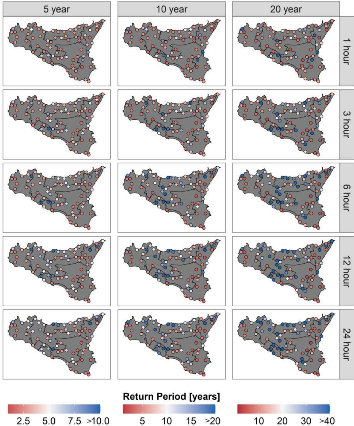
Figure 2.20: Spatial representations of the T_{SIAS} for the 72 considered SIAS rain gauges. Results are expressed for all reference durations (rows) and the T_{reg} of 5, 10, and 20 years (columns)
