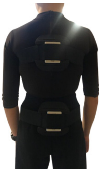
Figure 1. Method of placement of accelerometers with gyroscope
