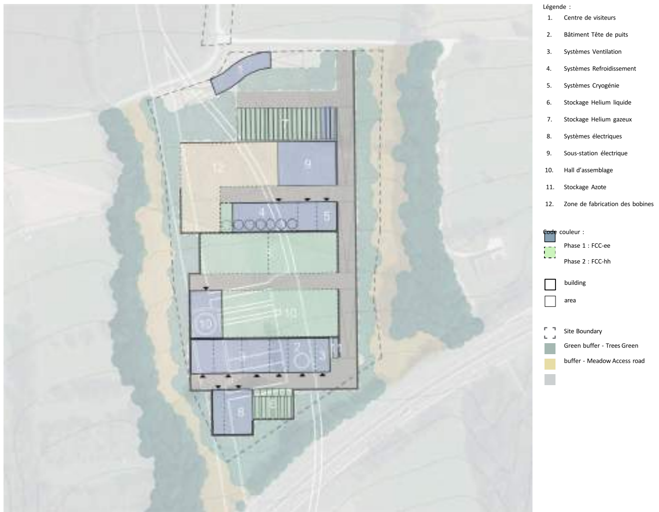
Fig. 2.70 Space requirements for a site integration of experiment site PJ in Dingy-en-Vuache and Vulbens, France. The architecture toolkit suggests centring the site between existing tree lines to ensure that functional fauna corridors are created. Compared to today, they can lead to an improvement of the habitat conditions
