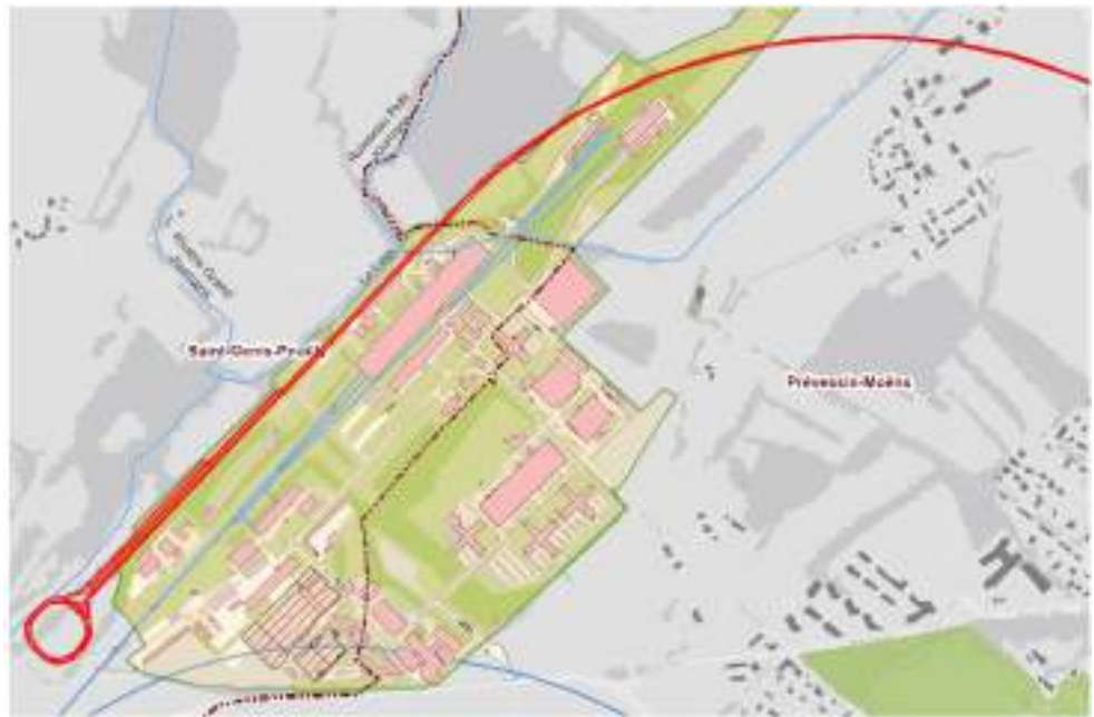
Fig. 2.48 Sketch of the current working hypothesis for a linear-accelerator based injector that has a length of about 1.2 km. A definitive placement remains to be developed in the frame of a design phase, considering environmental, existing experimental facility, territorial development and engineering constraints
