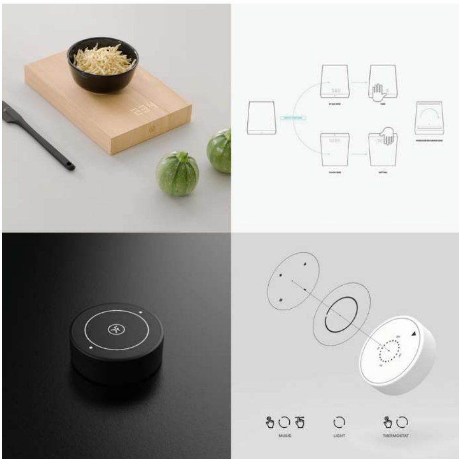
Fig. 2. Above, Slab! functioning as a kitchen scale and how it becomes a timer when reoriented. Below, Knob! and its multiple interfaces, which surface according to the positioning and interaction with other objects - the case is discussed in the next paragraph.
