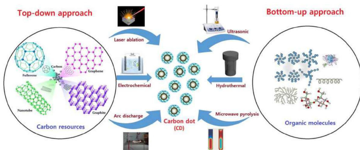
Figure 1.6: Schematic representations of different synthetic approaches for CD. [Adapted from [33]].
