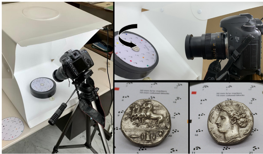
Fig. 10. In situ photogrammetry set-up including: Canon EOS 7D camera fixed on a tripod, macro lens (Leitz Leica, 1:2.8/60mm), automatic turntable, lightbox, printed markers.
