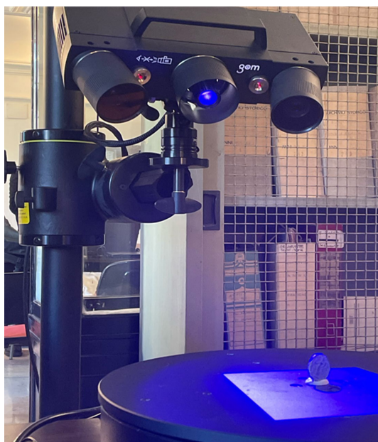
Fig. 9. Laser scanner Atos Q by GOM (Zeiss) used in combination with a tripod and the GOM ROT 350 rotation table inside the Salinas Museum.
