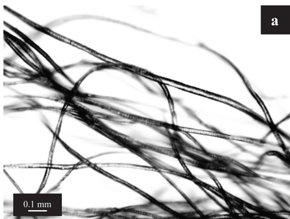
Fig. 6. Optical Microscope images of wool yarns wool sample treated with Hal/Keratin dispersion (R Hal:K = 0.5) before (a) and after (b) UV exposure.
