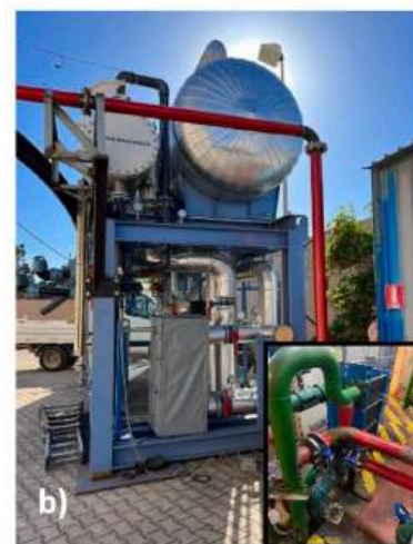
Fig. 2. A) block flow diagram of the heat input section of the med prototype plant. b) picture of the inlet heat exchanger and flash drum (inset showing the connection with the engine cooling circuit for waste heat recovery).
