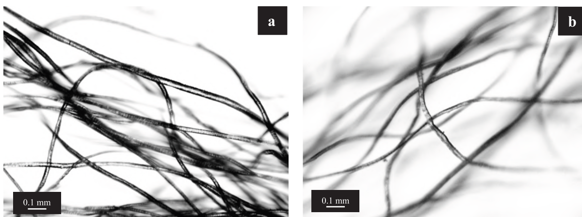
Fig. 6. Optical Microscope images of wool yarns wool sample treated with Hal/Keratin dispersion ( R_{\text{Hal:K}} = 0.5 ) before (a) and after (b) UV exposure.
