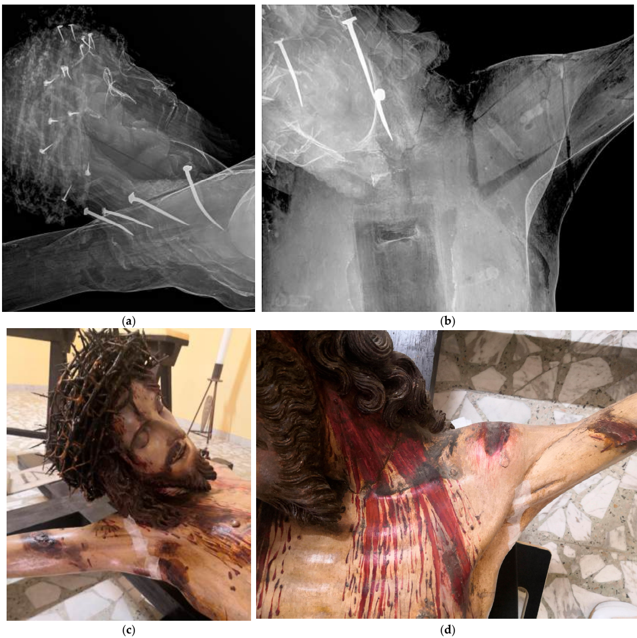
Figure 5. X-ray images of the Christ Crucified of Cutro and comparison with photographic images: head, upper part of torso, and right shoulder acquired on a (a,c) 45° oblique projection and an (b,d) antero-posterior projection. At the end of the nose, more visible in the oblique projection, a thin metal wire supports the tear probably made of wax or other natural resin.
