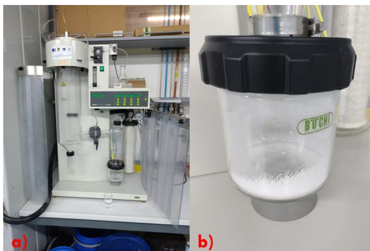
Figure 5-5: a) Image of the Mini Spray Dryer B-290 used during the experimental campaign and b) the close-up of the end-process collection vessel.
