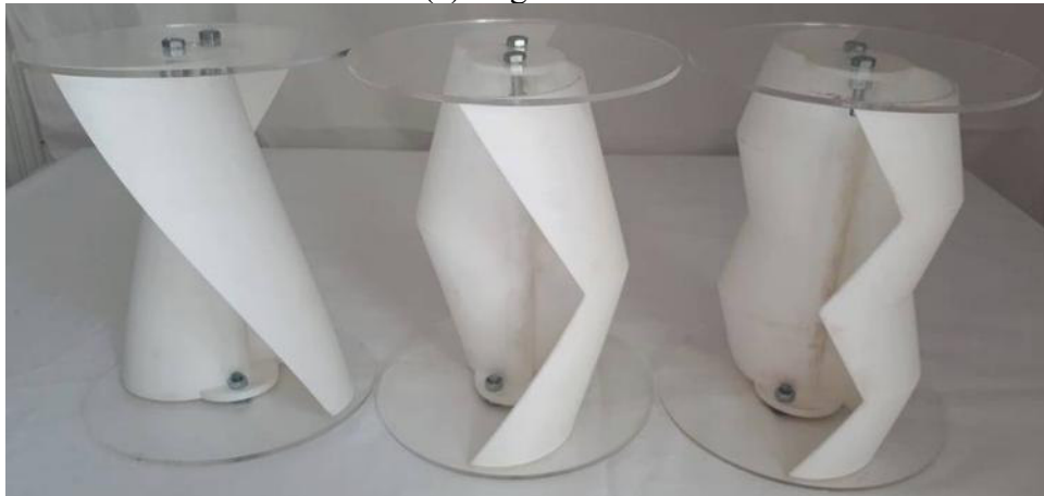
(b) 3D printed rotors
