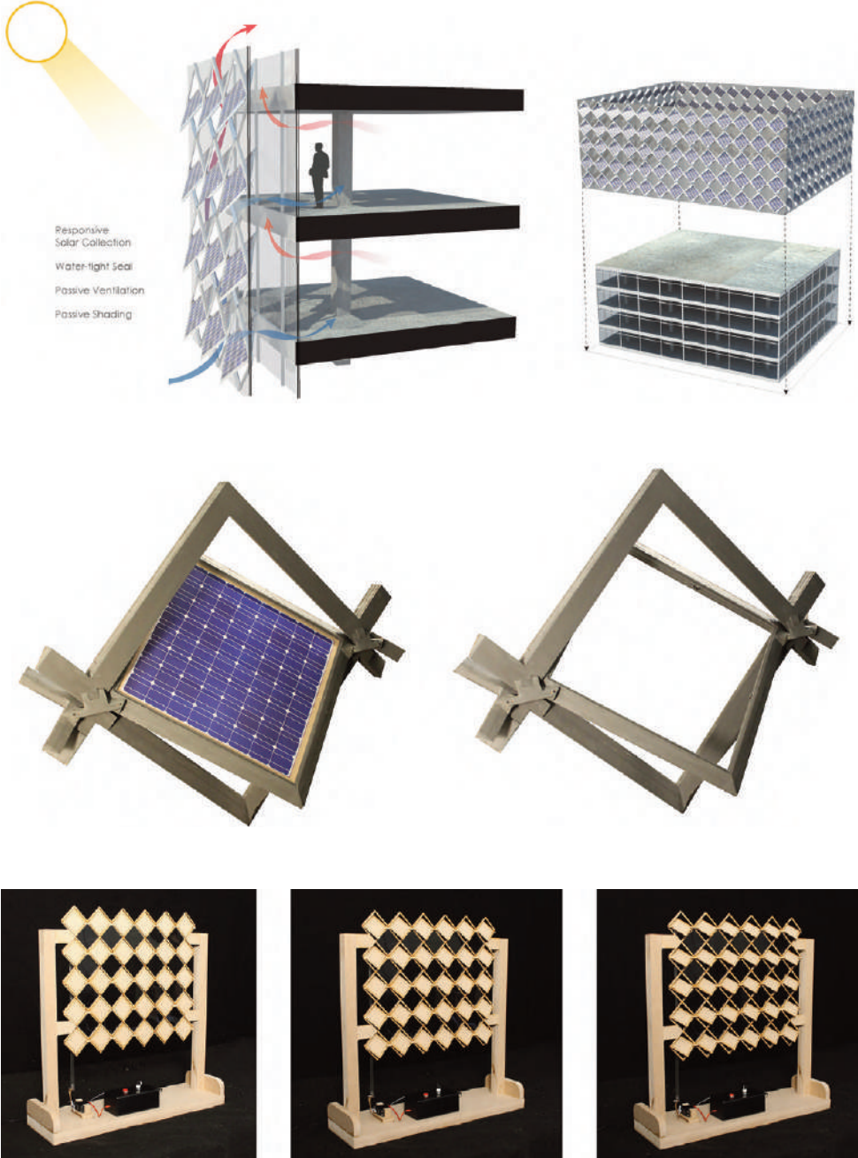
Fig. 4 | Adaptive Sola Skin, self-supporting solar collection façade: prototype with removable panel (credits: danielraznick.com/about/adaptive-solar-skin/ ).
