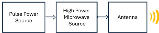
FIGURE 1. High Power Microwave (HPM) schematic block system.
