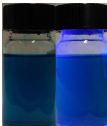
Figure S4.1 Photograph of a methanolic solution of NCND-ZnPc in daylight (left) and under UV light (365 nm) illumination (right).
