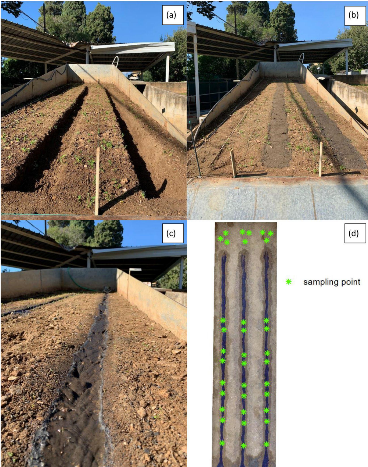
FIGURE 1 | View of the experimental plot with the two empty (a) and filled trenches (b), the preferential paths (c) and scheme of the sampling points (d).
