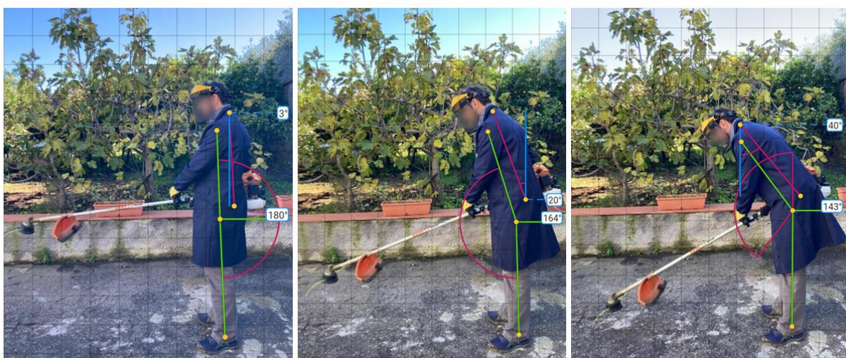
Fig 5: Explanatory image of the postural analysis of the working posture in the upright position (a), slightly forward inclined (b), and excessive forward inclination (c).
