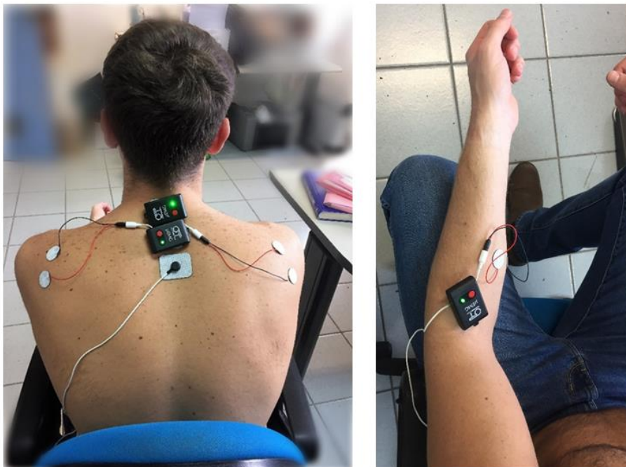
Fig 2: sEMG application over the neck and shoulders (a), and the forearm (b).
