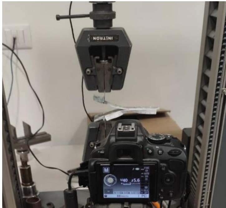
Fig. 100: Experimental DCB test setup.
