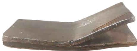
Fig. 116: Typical fracture of FML specimen with titanium alloy subjected to SBS test.
