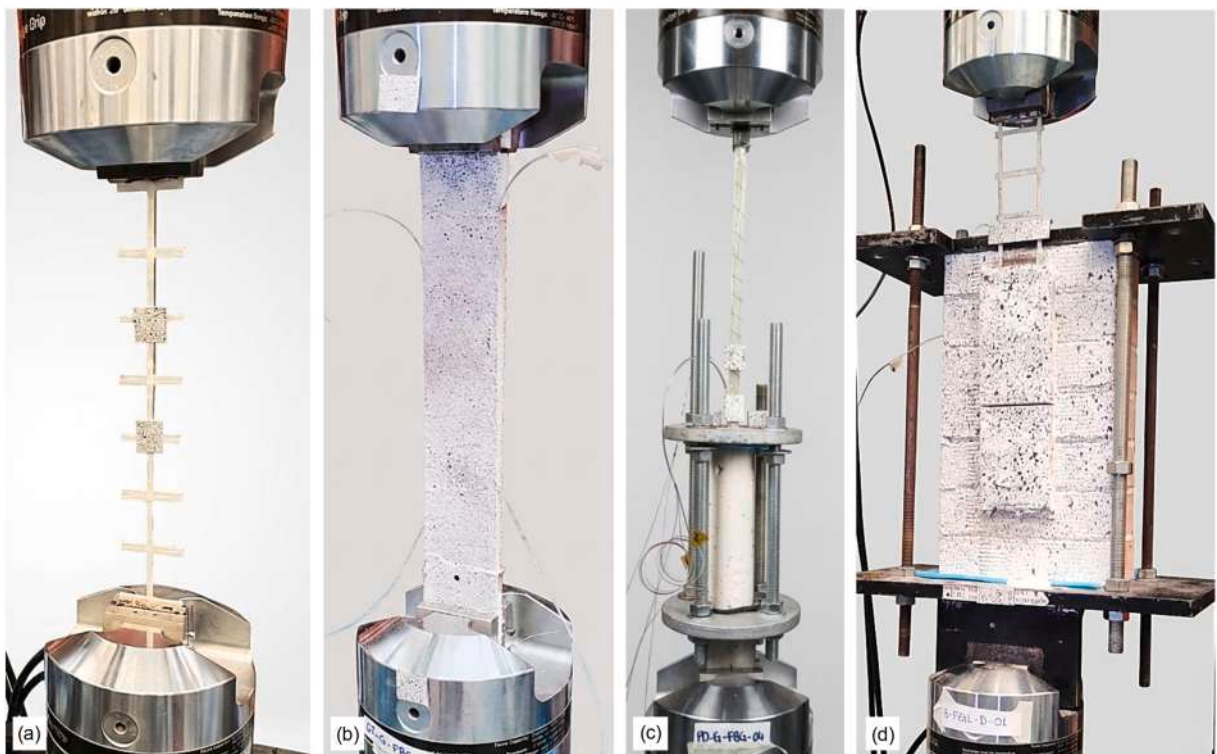
Fig. 2. Experimental setups of direct tensile tests on mesh bundles (a) and CRM coupons (b), of pull-out tests (c), and of shear bond tests (d).
