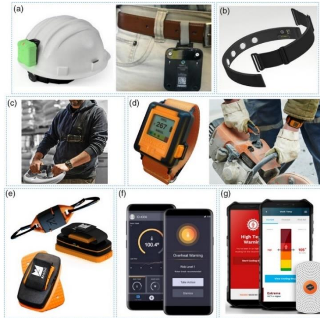
Figure 1.9: Examples of wearable devices for occupational safety monitoring. a) Smart helmet for monitoring safe working distance and interactions. b) Smart Cap measures brain waves to estimate alertness and fatigue level at work. c) Smart skeleton helps with heavy lifting by transferring the load from the upper body and back to the legs. d) Smart bracelet for the risk management of hand arm vibrations. e) Smart dynamometers to evaluate muscle strength and endurance. f) Smart PPE for safety monitoring of workers by tracking the microclimate, core body temperature, heart rate and exertion. g) Smart system for monitoring the work temperature of frontline workers [29].
