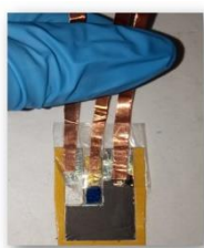
Figure 3.6: Photo of electrochemical sensor after PB electrodeposition on WE.
