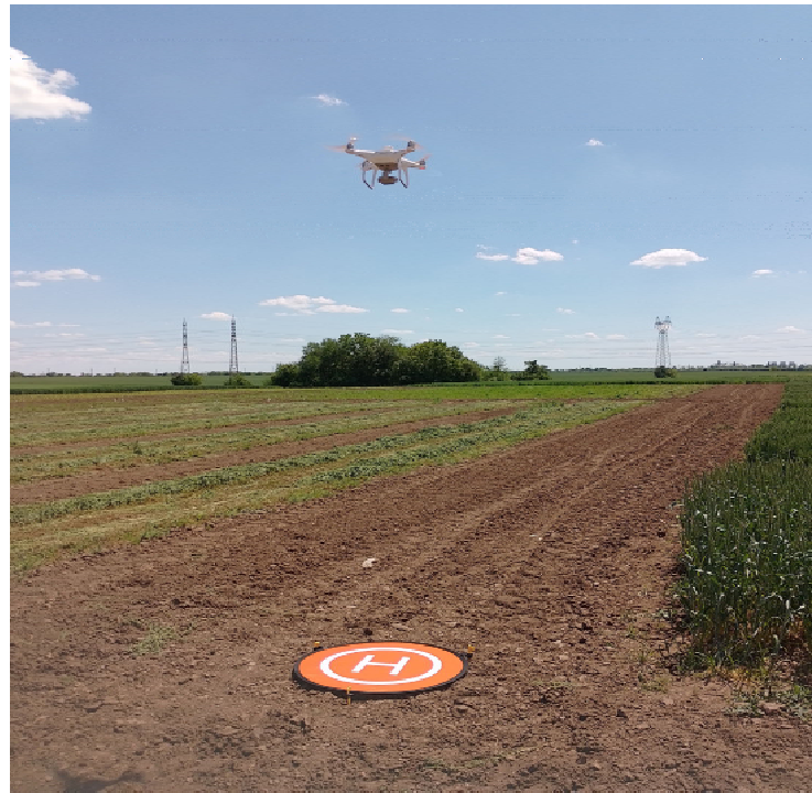
Figure 2. DJI Phantom 4 Multispectral unmanned aerial vehicle (UAV).
