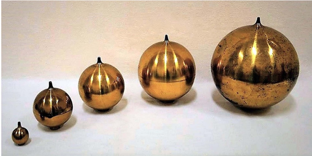
Figure 2. Historical Helmholtz resonators of different diameter D , from the Historical Collection of Physics Instruments of Palermo University ( D_1 \approx 4 cm, D_2 \approx 10 cm, D_3 \approx 13 cm, D_4 \approx 17 cm, D_5 \approx 23 cm).
