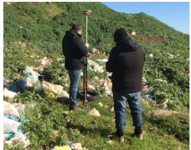
Figure 7. GNSS survey of the aluminium targets.
