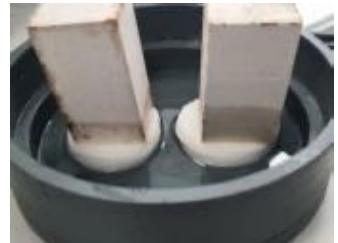
> 6.4 Water absorption by capillarity.
