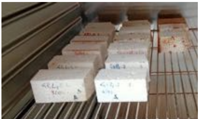
> 6.4 Water absorption by capillarity.
