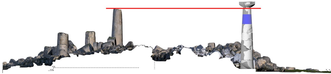
Fig. 14 - The section view supports the comparison between the height of the reconstructed column and the height of the 'Fuso della Vecchia'.
