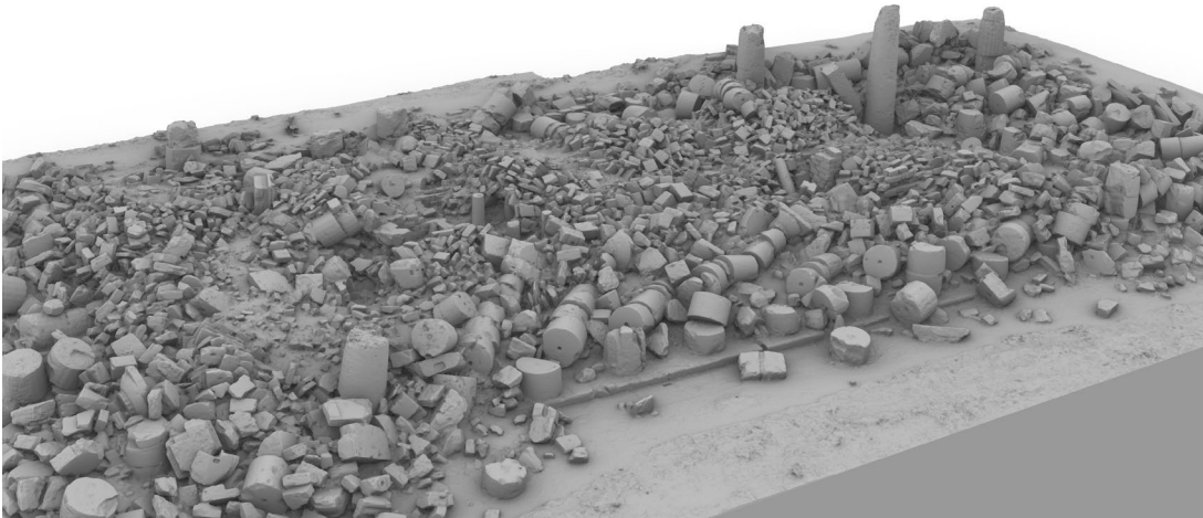
Fig. 7 - Perspective view of the 3D mesh generated with photogrammetric tools.
