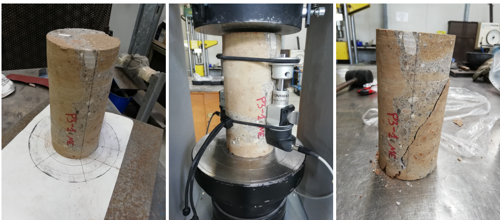
Figure V.15: Test configuration for determining the elastic modulus of ARC cylindrical specimens with diameter-to-height ratio close to 1:1 (specimen P3-1 ME).
