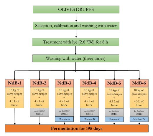
**Figure 1.** Experimental design for green table olive manufacturing. Abbreviation: <sup>o</sup>Bé, Baumè degree; NdB-1 and NdB-2 codes refer to the control trials; NdB-3, NdB-4, NdB-5, and NdB-6 codes refer to the experimental trials; *L., Lactiplantibacillus*.
