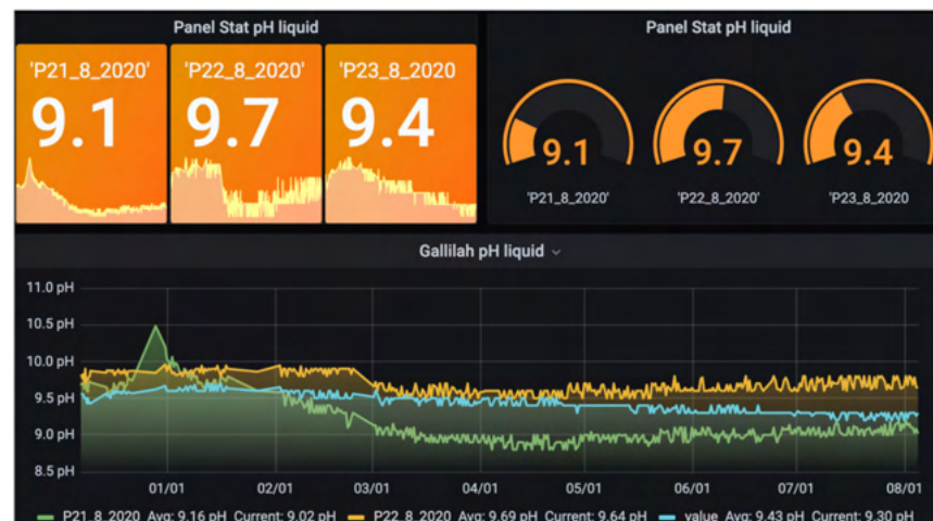
Figure 15. Grafana dashboard for real-time data visualization: pH concentration in the monitored concrete abutment.
