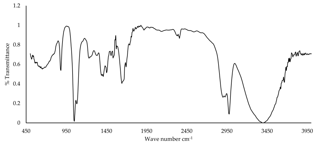
Figure 3. FTIR spectra for collagen extracted from different bluefin tuna waste tissues.
