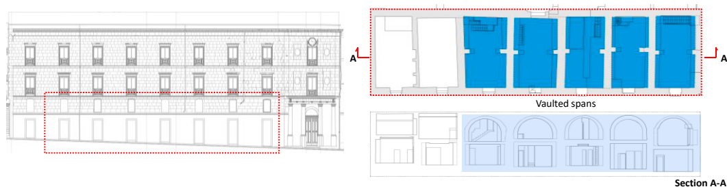
Fig. 5. Case study test building: main façade, extracted plan and section of the vaulted spans at the mezzanine floor.
