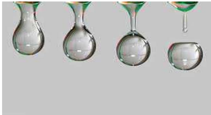
Fig. 22: A picture showing some phases of the process leading to drop formation from a capillary tube or dropper. The drop breaks when its neck can no longer bear its weight.
