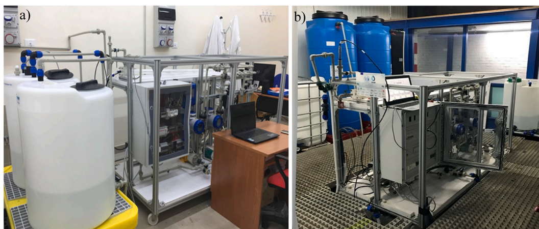
Fig. 5. A picture of the novel proprietary crystallization reactor tested at the Brine Excellence Center laboratory of University of Palermo (a), then installed and operated at the premises of Plant One (Botlek, Rotterdam, NL) (b).
