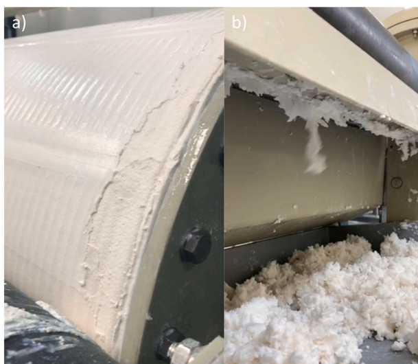
Fig. 7. a) Magnesium cake on the filter cloth surface and b) detached magnesium hydroxide in the collection tray.
