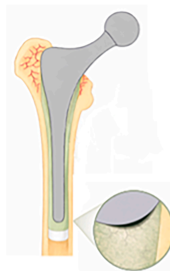
Fig. 1. Schematic representation of femoral stem subsidence within the cement mantle, illustrating the generation of radial stresses at the bone–cement interface that may contribute to the development of Vancouver type B2 periprosthetic fractures.
