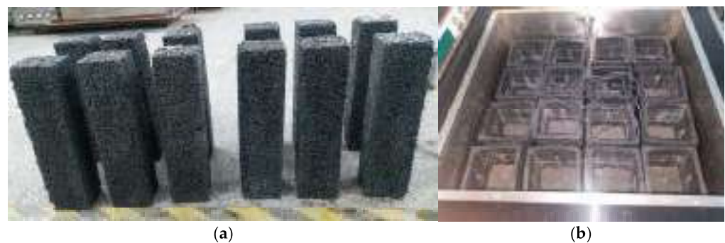
Figure 3. Specimens prior to (a) and during (b) freeze–thaw testing under saturated conditions.
