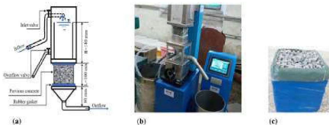
Figure 2. Permeability test: (a) test set up; (b) NELD-PC370 tester; (c) specimens laterally wrapped.
