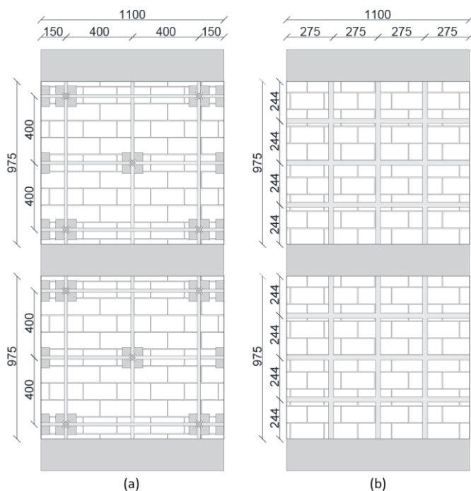
Figure 8 Geometrical configurations of the retrofitted walls: (a) CAM® system and (b) steel grids
