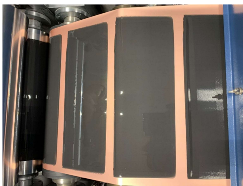
Figure 8 – Anode coating on roll-to-roll machine
