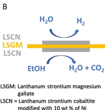
Figure 1: Features of the fully perovskite electrolyte-supported cell used in this experiment and expected reactions
