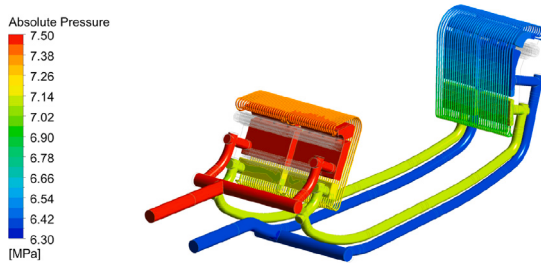
Fig. 7. VT cooling circuit absolute pressure field distribution.
