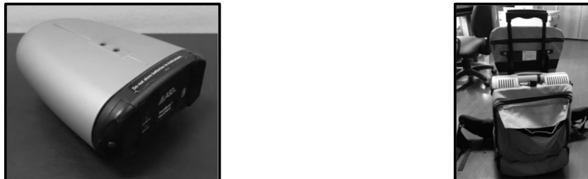
Figure IV Spectroradiometers a) from 325 to 1075 nm and b) up to 2500 nm
