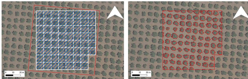
Figure 5.4 Example of a Sentinel-2 grid fully contained within the field perimeter (left) and the intersection of the grid with the field perimeter (right)
