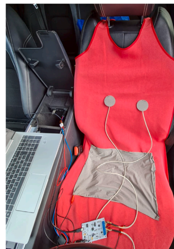
Fig. 14. Capacitive electrodes integrated into the car seat cover.
