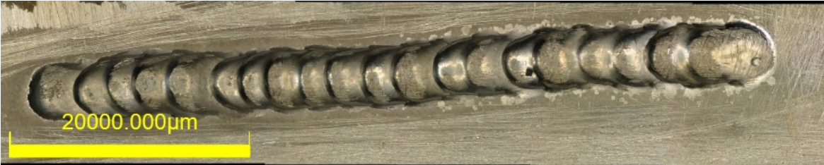
Figure 19. extruded wire deposition in the WAAM process.
