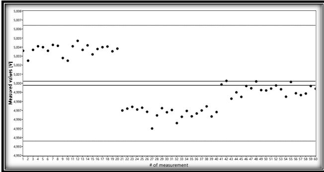
**Fig. 5.** Voltage RMS values measured by using three NI USB 9008 DAQ
