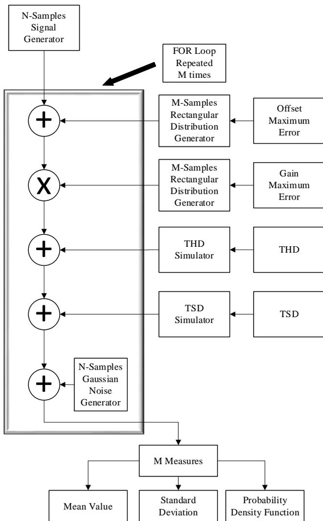
Fig. 1. Flow diagram of the simulator
