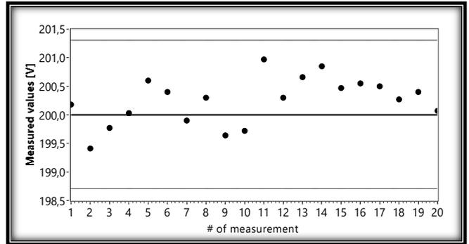
**Fig. 6.** Voltage RMS values measured by using the NI USB 9225 DAQ in proximity to a power drive system
