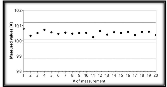
**Fig. 4.** Current RMS values measured by using the 0,1  $\Omega$  shunt and the NI USB 9239 DAQ
