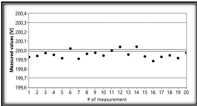
**Fig. 3.** Voltage RMS values measured by using the NI USB 9225 DAQ
