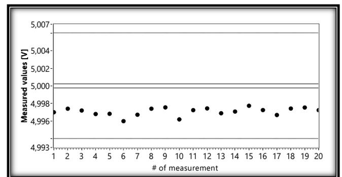
Fig. 2. Voltage RMS values measured by using the NI USB 9239 DAQ
