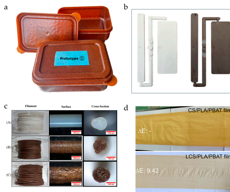
Figure 11. Prototype of biodegradable food containers (a) and biocomposites samples (b) obtained for injection molding; biocomposite filament for 3D printing applications (A) pure PBS, (B) PBS/10%CBS, (C) PBS/20%CBS (c); biocomposite film for food packaging applications (d). Reprinted (adapted) with permission from [67,77,87,91].
