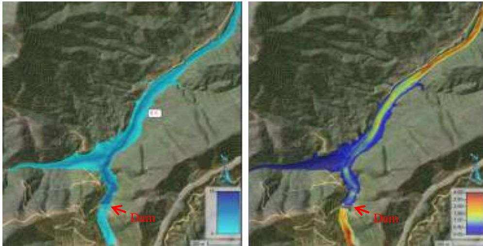
Figure 15 Maximum water depths (left, in m) and velocities computed with HEC-RAS (right, in m. s -1 )
