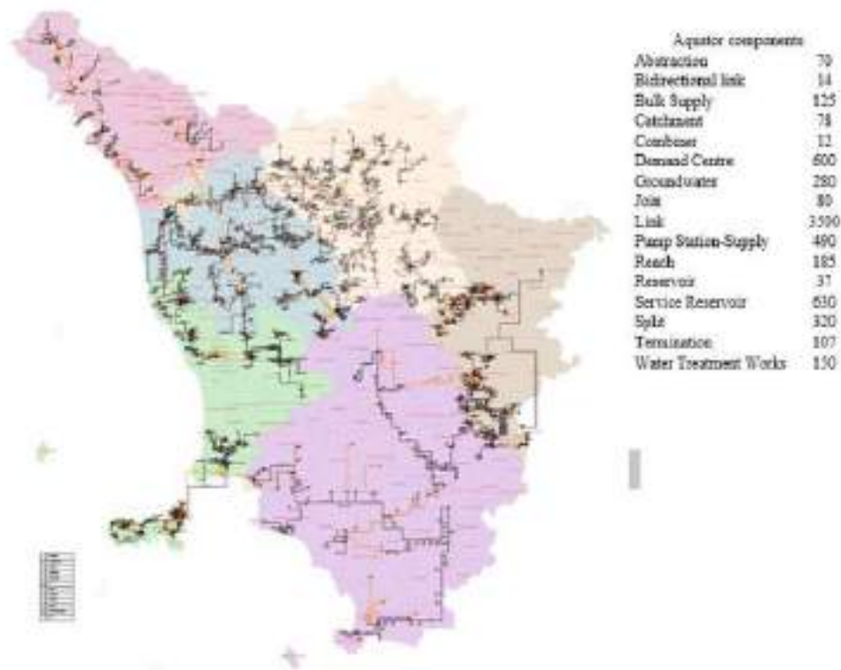
Figure 1 Water supply systems of the seven Tuscan utilities modelled with Aquator (different colours indicate the areas operated by different water utilities) and summary of the number of components.
