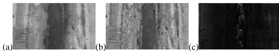
Figure 8 Platani river case: application of (a) grayscale, adding (b) CLAHE, or (c) intensity capping filters.
