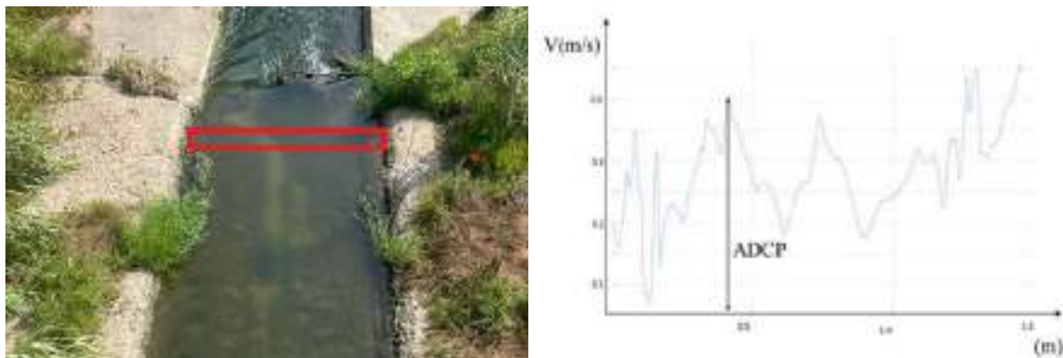
Figure 2 Comparison of velocity determined by image analysis with ADCP measure
