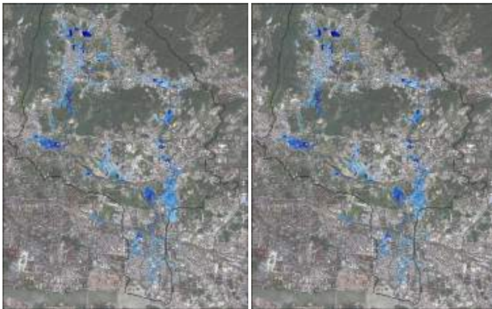
Figure 1. The simulated inundation water depth predicted using the CNN model (left) and the coupled model (right) under 50a test rainstorm scenarios ( t=2.0h ).
