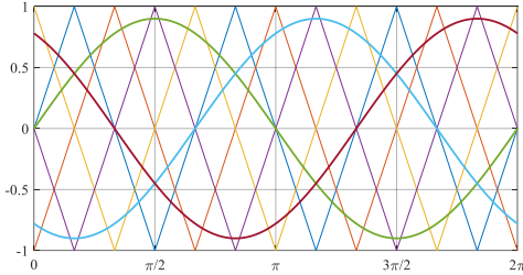
Fig. 2. Phase Shifted Pulse width Modulation scheme.
