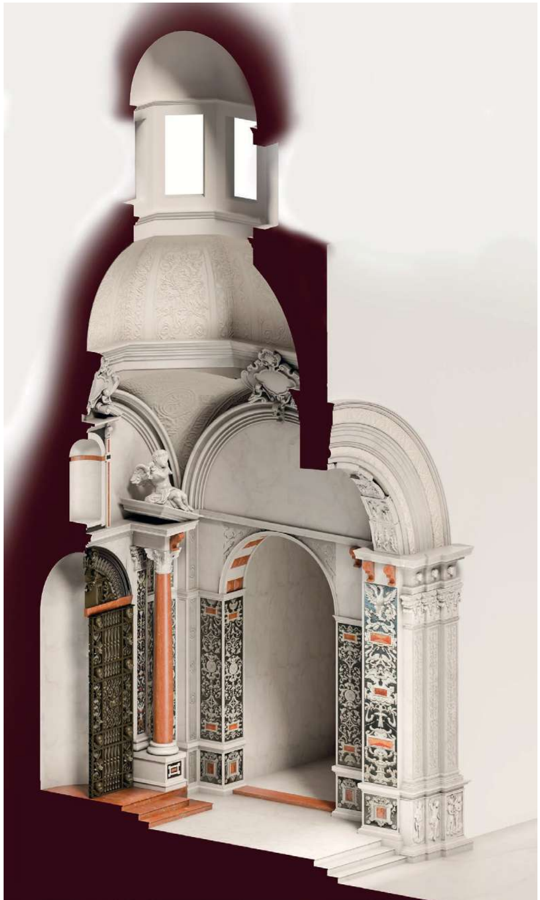
Fig. 10. Axonometric cross-section of the digital model of the chapel of saint Rosalia (elaboration by the authors).
