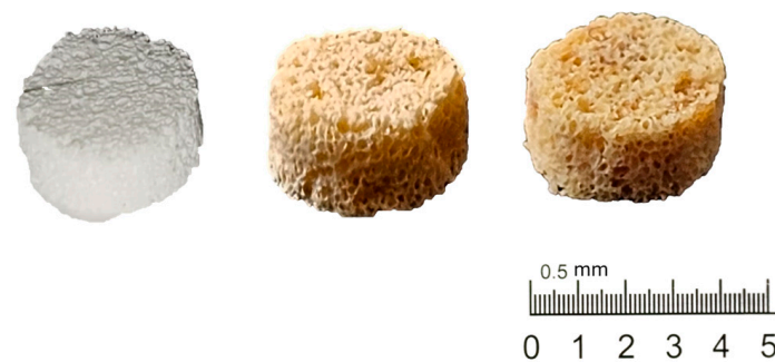
Figure 2. Digital images of samples, right to left: PLLA, PLLA-RA 2%, and PLLA-RA4%.
