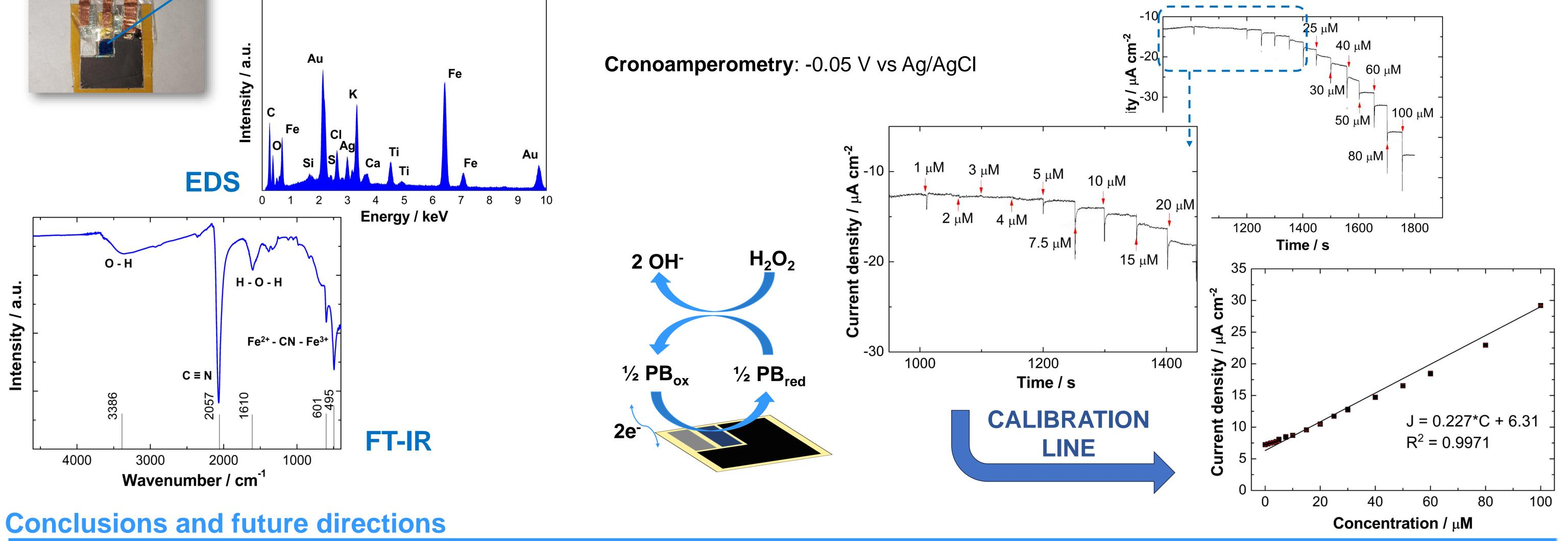
This study reported the development of a wearable sensor for detecting  $H_2O_2$  in exhaled air. A linear range from 1 to 100  $\mu$ M was obtained with a sensitivity of 0.227  $\mu A\mu M^{-1} cm^{-2}$  for liquid phase.
