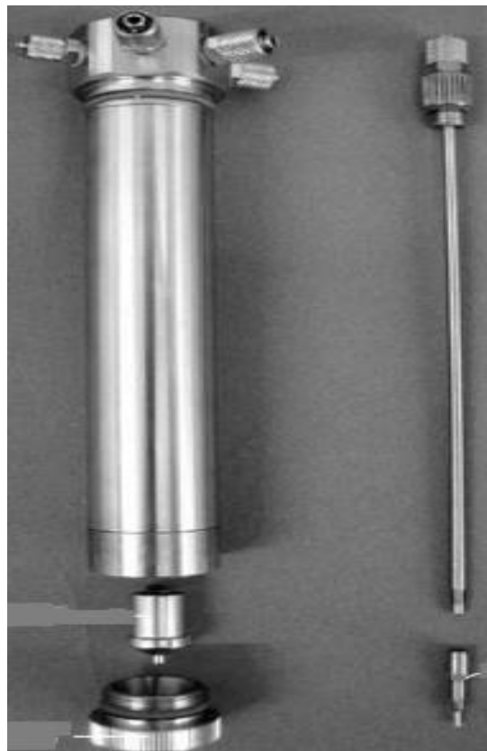
Figure 13 Pneumatic or multi-phase nozzle (Mini Spray-Dryer Buchi B-290).
