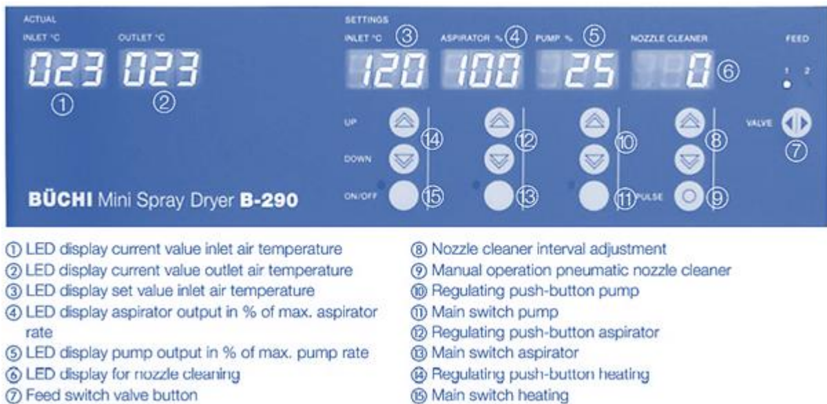
Figure 15 Description of the control elements display of the Mini Spray-Dryer Buchi B-290.
